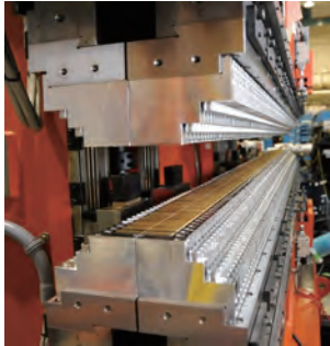
Fig. 3. New U5 undulator and beam duct just before installation (upper) and new magnet configuration (lower).
